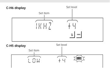
• Each frequency band can be adjusted in the range between -4 and +4.
